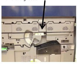
**7.** To remove the old drum cartridge, stand on the left side of the Drum Cartridge Drawer.
