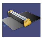
**6.** Grab the **Release Handle** and pull the Drum Drawer straight out.
