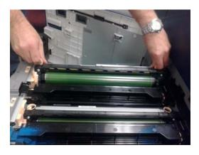
**9. Simultaneously** press down on both ends of the drum cartridge to **horizontally** place the drum cartridge into position.
