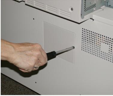
3. Pull out and remove the Suction filter cover.
