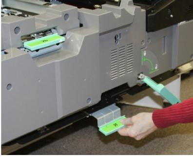
8. Locate and lift up on the 2e lever to remove jammed paper.
