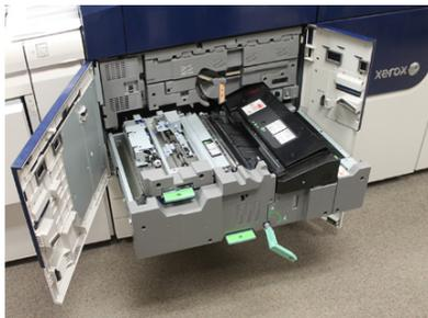
4. When the Fuser has cooled, pull the Transfer Drawer out to the jam clearance position.
