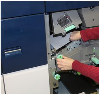
4. Rotate the **5d** knob clockwise to advance paper and pull down on the **5c** green lever to remove any paper in this area.
