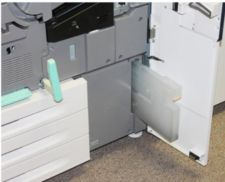
3. Grasp the handle of the Dry Ink / Toner Waste Bottle and pull it halfway out of the press.
