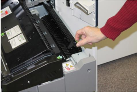
9. Lift up the 2d Lever to remove jammed paper.
