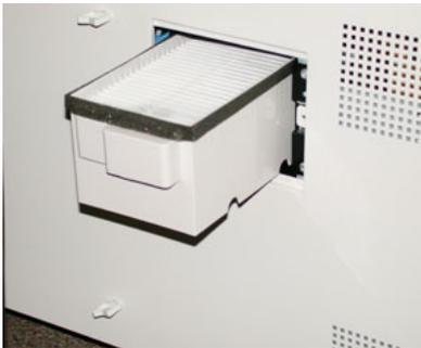
5. Remove the Suction filter out of the box.
