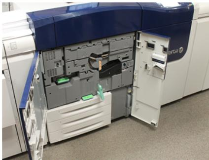
3. Unlock and pull out the Transfer Drawer by turning the green **2** handle (at the center) to the right until it is in the horizontal position. Pull the drawer straight out until it stops.
