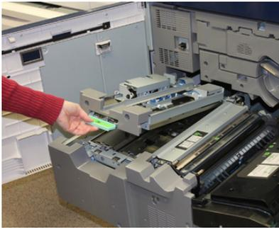
5. If paper is jammed at the top of the Transfer Module, remove paper from the registration roll (area **2a**) by pulling it straight out.
