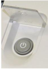
Use the Power On / Off button to power **ON** or power **OFF** the press.
