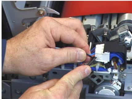
10. Locate the storage area of the press that holds the pack of Fuser and Pressure Roll Lift Handles. Remove the Lift Handles pack from the storage area.
