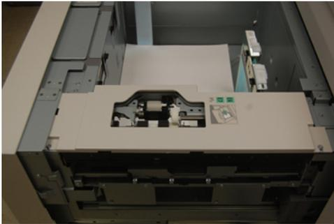
3. Remove the nudge roll by pushing down on the black tab with one hand (which raises the roll upward) and then squeezing the metal shaft on both ends with your other hand. Lift out the nudge roll.
