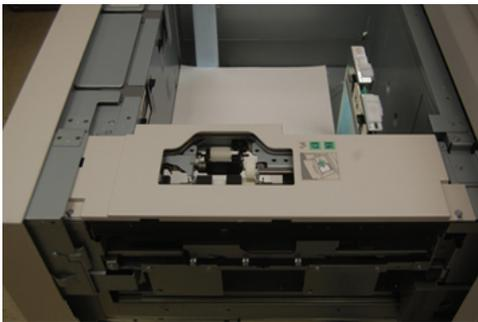
Chained (Second) Oversized High Capacity Feeder (OHCF / Trays 8 and 9)
