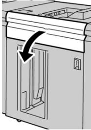
2. Lift the green handle(s) and/or rotate the green knob and remove all paper in the entrance area.
