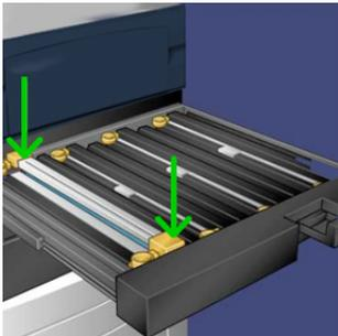
10. Immediately close the drum cartridge drawer to protect the other drums from light.
