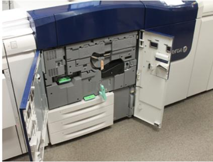
3. Unlock and pull out the Transfer Drawer by turning the green **2** handle (at the center) to the right until it is in the horizontal position. Pull the drawer straight out until it stops.
