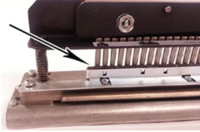
3. To oil the die set, apply a small bead of oil along the entire length of the felt strip that is located on the die set.
