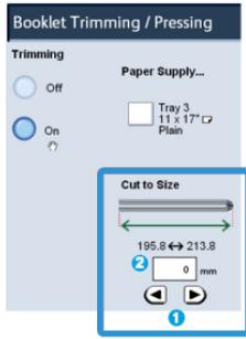
1. Select the arrow buttons to decrease or increase the trimmer setting. Adjustments are made in 0.1 mm/0.0039 inch increments.
