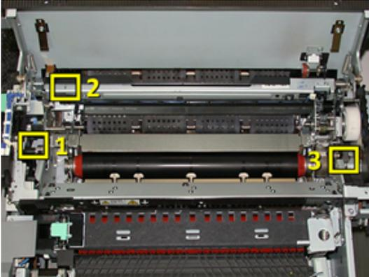
1. Place the Fuser Belt Module Handles on each side of the belt and reinsert the required Fuser Belt Module into the Fuser Assembly.
