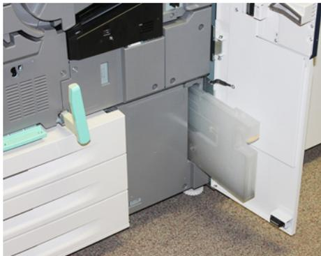
3. Grasp the handle of the Dry Ink / Toner Waste Bottle and pull it halfway out of the press.
