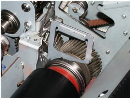
4. Install the new Pressure Roll Assembly. Use the Pressure Roll Handles to help position the Pressure Roll in the Fuser Assembly.
