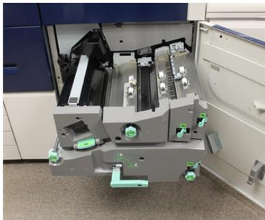
7. Rotate the 4a knob clockwise and advance paper to remove.
