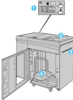
1. **Control Panel:** Provides manual control of the various HCS functions.
