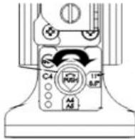
5. When the arrows align, release the **Die Stop Knob**.
