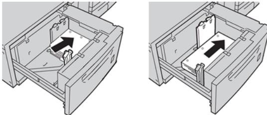
7. Adjust the paper guides by pressing in the guide release and carefully moving the Edge Guide until it lightly touches the edge of the stock in the tray.
