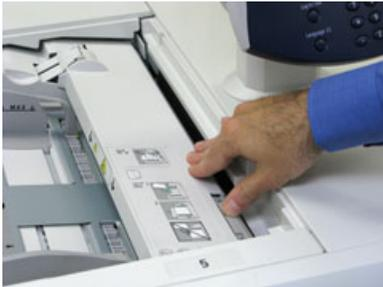
5. Pull open the (OHCF) **Top Drawer** (located at the top of Trays 6 and 7).
