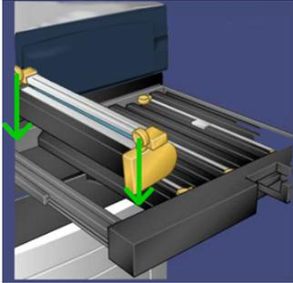
9. Press both ends of the drum cartridge to place it in a horizontal position.
