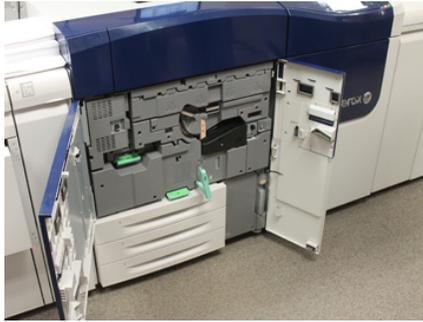
3. Rotate and turn the R1-R4 Drum Drawer Handle to the unlock position.
