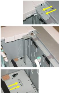
6. Tighten the thumb screw so it locks the Postcard Bracket in place.
