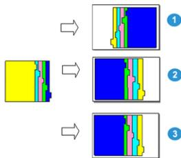
1. If using the optional HCF (letter-size / A4) or the OHCF, load the tabs upside down and change the order one by one (as shown in the illustration).
