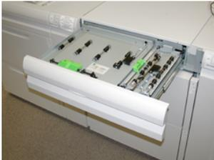
6. Lift levers **2a** and **2b**, and remove any paper jams.
