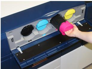
4. Remove the dry ink / toner cartridge by slowly and gently pulling it straight out. While pulling out, hold the bottom of the cartridge with your other hand to give it support.
