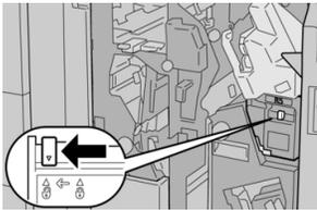
4. Hold R5 as shown in the figure and remove the staple waste container from the press.
