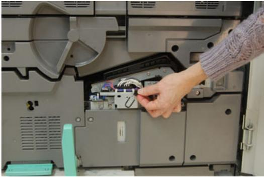
8. Position the fuser cover back on the assembly and screw tightly in place.
