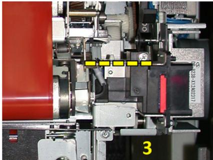
Make sure the fuser is seated correctly and completely or the Fuser Top Cover will not close and machine damage may result.
