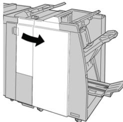
3. Pull out the folder output tray (2d), swing lever 2e/2f to the right, and remove the jammed paper.
