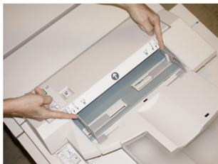
3. Load the paper or tabs, aligning it to the front side of the tray.
