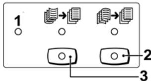
1. **Auto** button: When this indicator is lit, the appropriate curl correction is automatically performed depending on the sizes and orientation of the printed output. The button should be set to Auto for most situations. The button automatically switches to the Auto mode when:
