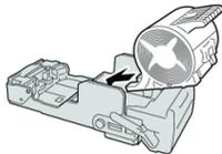
6. Reinstall the cartridge unit to its original position in the finisher.
