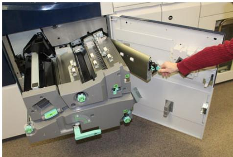
9. Grasp the green Drawer handle (**4**) and gently push in the Exit Drawer assembly completely. Rotate the handle to the left to lock the drawer in place.
