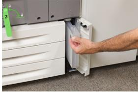
4. Grasp the handle of the Dry Ink/Toner Waste bottle and pull it halfway out of the press.
