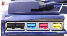
2. Lay paper on the floor before removing the cartridge. This will allow any excess dry ink/toner to fall on the paper.
