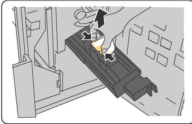
4. Dispose of the staple cartridge according to the instructions contained in the new staple cartridge box.
