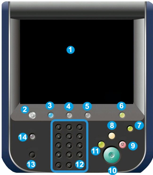
1. **Touch Screen.** The touch screen allows you to select all the available programming features. It also displays fault clearance procedures and general machine information.
