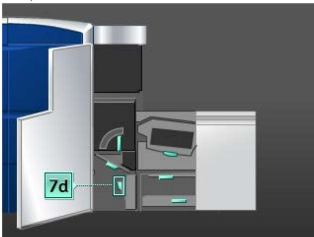
9. Use a damp, water-moistened (not wet), lint-free cloth to clean the paper path only in the green lever jam clearance areas as shown in the illustration.
