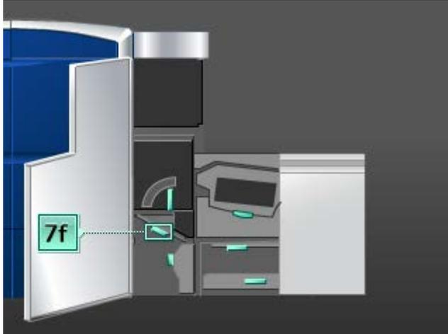
6. Use a damp, water-moistened (not wet), lint-free cloth to clean the paper path only in the green lever jam clearance areas as shown in the illustration.
