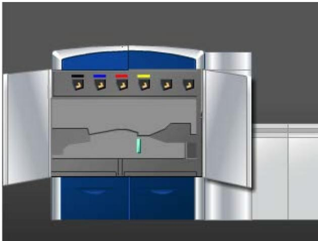
2. Use a damp, water-moistened (not wet), lint-free cloth to clean the paper path only in the green lever jam clearance areas as shown in the illustration.
