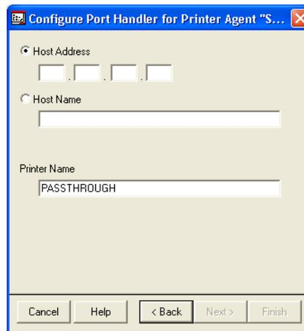
If you select the Host Address field, type the IP address of the EFI Splash RPX-iii.
