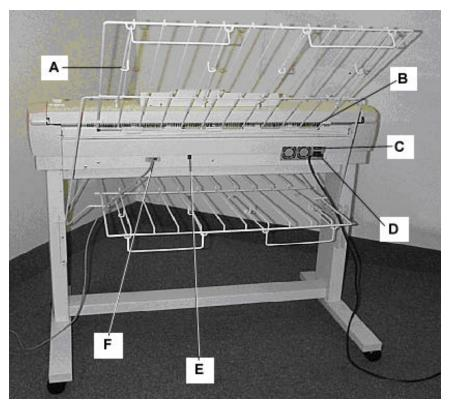
A: Standard StackerB: Document Exit SlotC: Power On/Off switch
