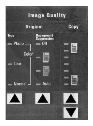
The SCAN SYSTEM firmware must be at version 3.0.9 or greater to support **Normal**, **Line**, **Photo**, or **Color** Type. If the SCAN SYSTEM is not at the required version an error message. Depending on what **Mode** is selected (COPY or SCAN) the message will be displayed as show below.
