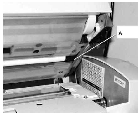
A: Calibration Roll Drive Gear
