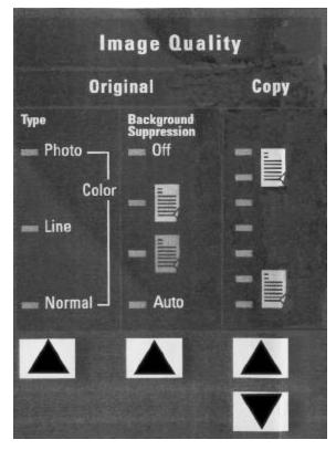
There are many settings. other than **Media Selection**, **Image Quality** and **Reduce/Enlarge** areas, available on the Control Panel. The Transform special features key allows you adjust the margins around the image, specify the position of the image on the media, and transform the image into a mirror and/or inverted. Refer to the applicable sections of this guide for detailed information about the many document settings available to you.
