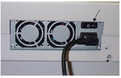
When the Scanner is switched on, the fluorescent lamp inside the Scanner illuminates immediately. If the lamp does not illuminate, refer to the "Problem solving" section of this guide.
