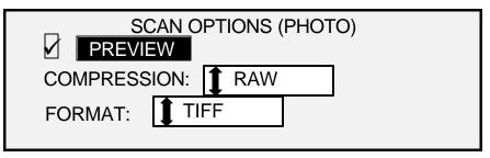
NOTE: The **Background Suppression** option cannot be used with the **Photo** setting. If **Photo** is selected, **Background Suppression** is automatically set to Off.
