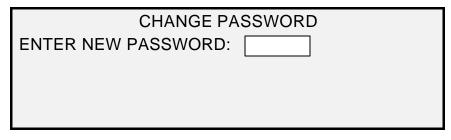
6. Use the numeric keypad to enter the new password. The password will display as asterisks.
