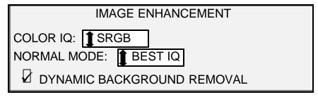
When enabled, the dynamic mode will monitor the whole document and adjust the image quality settings as the document is being scanned in order to optimize the background of the copy.
