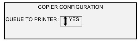
8. Press the **Enter** key to confirm the response. A status message is displayed indicating that the configuration has been queued to the Printer.
