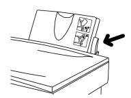
Note: E1 and E2 jams will occur if the release lever does not lock into place during paper loading.
