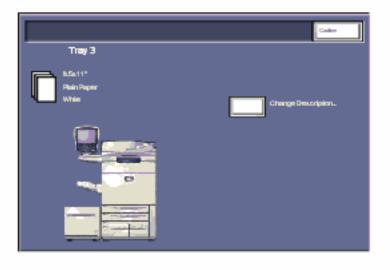
The tray settings are displayed on the touch screen. If the tray settings are correct, select the **Confirm** button. Alternatively change the paper type or color by selecting the **Change Description** button on the touch screen.
