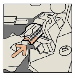
Unpack the new staple cartridge. Insert the new staple cartridge while gripping the orange lever until you hear it click into place. Close the front cover of the finisher.
