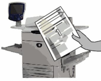
To ensure optimum print quality at all times, regularly clean the glass areas of your machine. This helps avoid output with streaks, smears, and other marks that transfer from the glass area when scanning documents.
