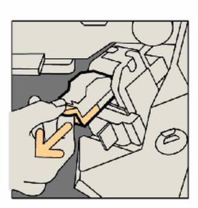
Hold the R1 lever of the staple cartridge. Hold the orange lever and pull the cartridge towards you to remove. Dispose of the staple cartridge according to the instructions contained in the new staple cartridge box.
