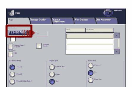
Type in the number of the receiving fax machine using the number keys on the keypad. The number will appear in the window indicated. Then add the number to the Recipient List by pressing the Add button.
