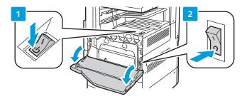
To restart printer, use the **secondary power switch** on top of printer. For full shut down turn off the **secondary power switch**, then turn off the **main power** switch behind front cover.
