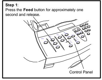
Figure 2. Pressing the Feed Button
