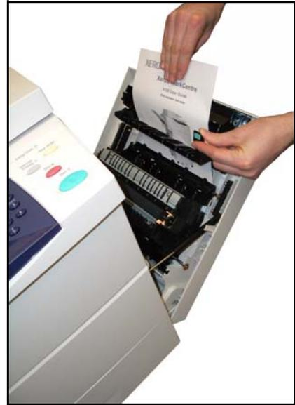
2. Ensure that all jam clearance handles and levers are returned to their correct positions.
