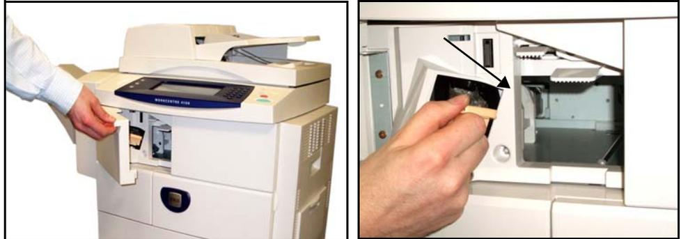
2. Pull on the latch to remove the staple unit.
