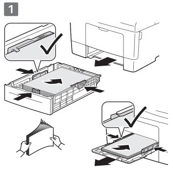
For best results, fan the edges of the paper. Adjust guides to fit the paper size. Do not load paper above the maximum fill line.
