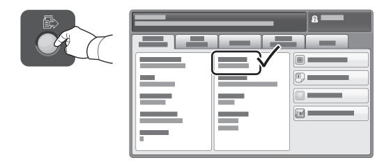
If the IP Address does not show in the upper left corner of the touch screen, press Machine Status and check the information field.
