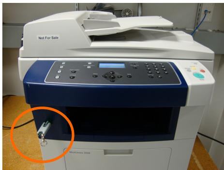
2. Press the **Up/Down** arrow buttons to highlight **Print from USB** and press **<OK>**. Your machine automatically detects the device and reads data stored on it.
