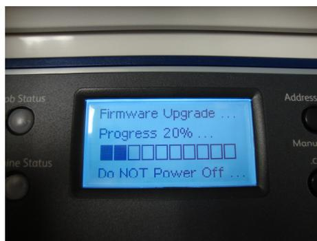
5. Once the upgrade is complete, you can remove the USB flashdrive. The machine will return to ready mode briefly, then reboot once, and return again to ready mode.
