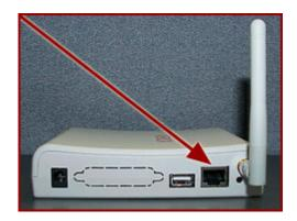
4. Connect the other end of the crossover cable to the Ethernet port on the computer that will be used to configure the adapter using an Internet browser.
