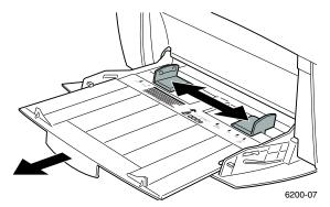
3. Insert the paper, transparencies, or envelopes in the Multi-Purpose Tray. Load the side to be printed *facedown* with the *top* of the page entering the printer *first*. Do not load paper above the fill line. Place envelopes with the *flap side up* and *top* of the envelope towards the right of the printer. (For A7 envelopes, place the *flap side up* but have the *top* of the envelope enter the printer *first*.)
