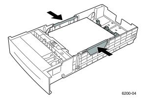
**6.** Insert the tray and push it completely into the printer.
