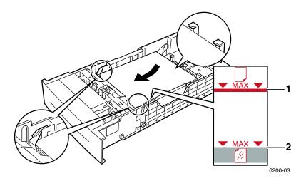
**5.** If necessary, push the width guides inward to match the size of the paper.
