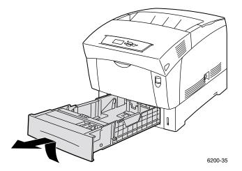
2. If loading paper having a different width, push the width guides outward. If loading paper having a different length, tilt the back guide forward, slide the guide, and insert the pins on the bottom of the guide into the holes in the tray corresponding to the paper size you are loading.
