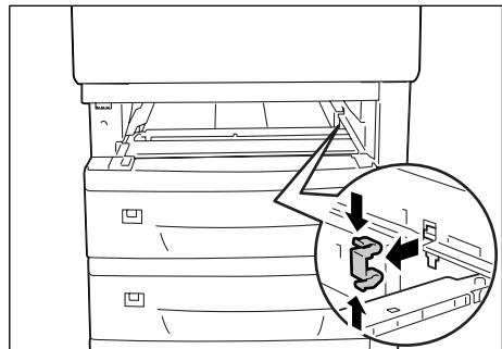
4. Release the upper tab of the clip on the inner left side of the printer. Tilt the tab towards the inside of the printer.
