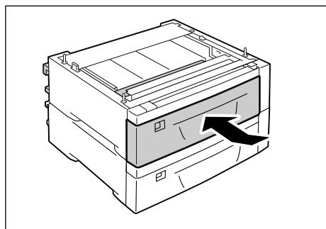
7. Repeat Steps 3 to 6 to install another sheet feeder on top of the two sheet feeders.
