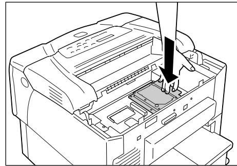
8. Hand-tighten the two screws (supplied) from the outside of the printer and secure the hard disk onto the controller board.
