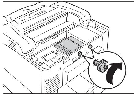
9. Re-attach the metal plate cover on the printer by tightening the three screws loosened in Step 4.
