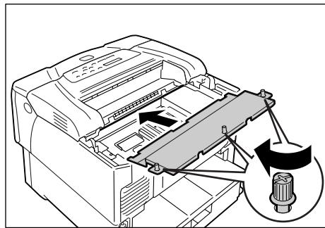
10. Re-attach the rear cover on the printer by tightening the two screws removed in Step 2.
