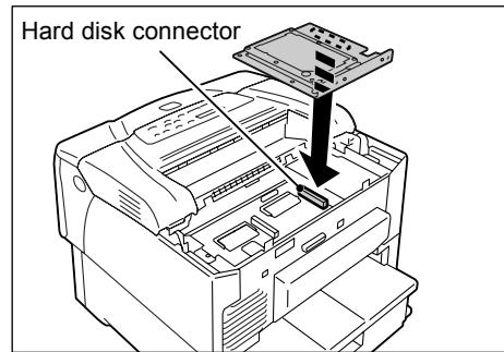
7. Press the hard disk as shown in the figure and firmly insert it into the connector.
