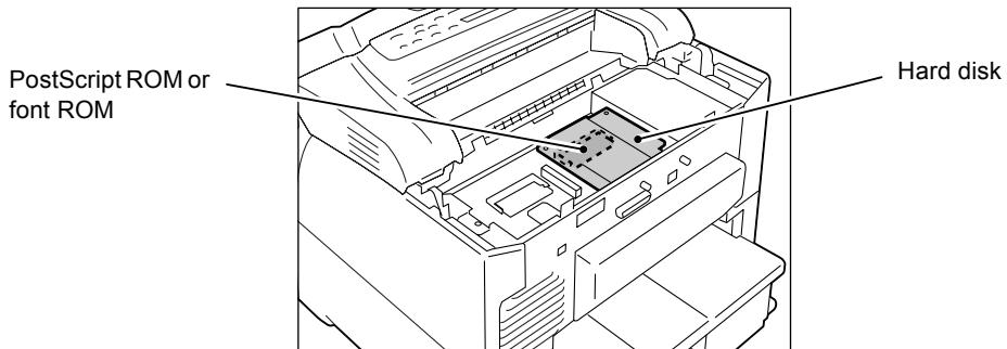
Follow these steps when installing the internal hard disk to the printer.
