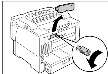
3. Remove the two screws that secure the rear cover to the printer.
