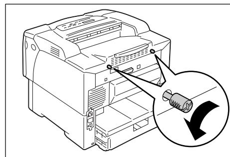
4. Pull the rear cover forward and remove it from the printer.
