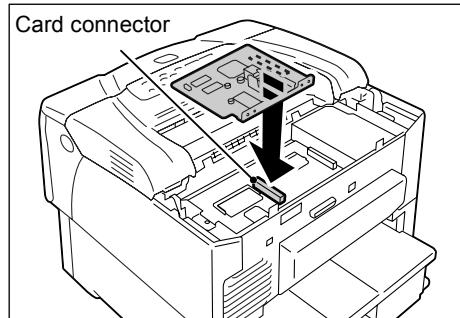
8. Push the network expansion card as shown in the figure and firmly insert it into the connector. You may need to wiggle the board slightly to get it to seat properly.
