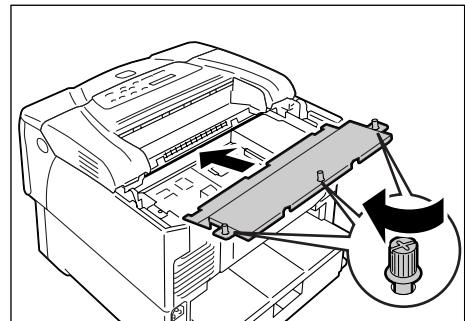
11. Re-attach the rear cover on the printer by tightening the two screws removed in Step 2.
