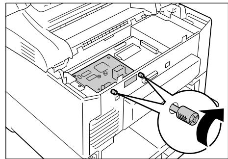
10. Re-attach the metal plate cover on the printer by tightening the three screws loosened in Step 4.
