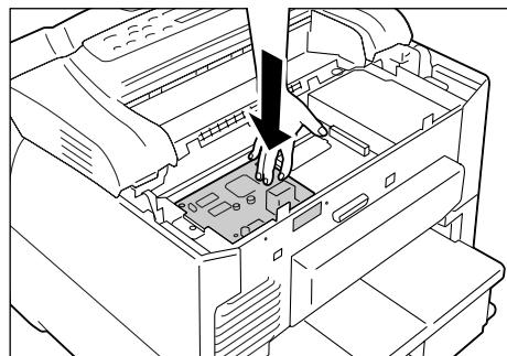
9. Secure the card by hand-tightening the two screws (supplied) on the outside of the printer.
