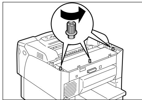
6. Pull the metal plate cover forward and remove it from the printer.
