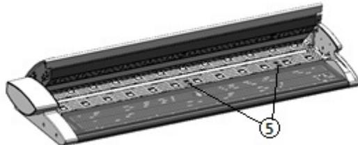
9. With both hands grasp each side of the Scanner Lid and lower it while depressing the lid latches on the underside of either end. Ensure that each side clicks into the locked position by pressing firmly on both ends.
