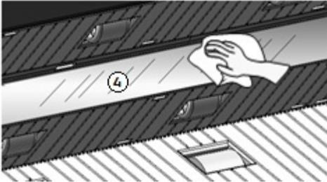
7. Wipe the Pinch Rollers and Feed Rollers with a water-dampened cloth.
