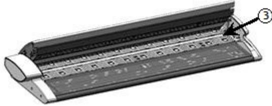
6. Wipe the Contact Image Sensor with a clean, dry, lint-free cloth. If the Scanner Contact Image Sensor (CIS) becomes dirty, image quality defects such as black lines or streaks may appear on scanned images.
