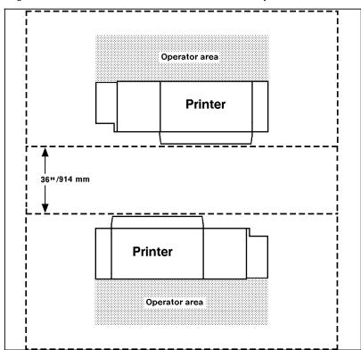
Figure 1-7 shows the two printers facing each other. The printers share 12 inches/305 mm of the general service space but not the exclusive operator area in front of each printer. Therefore, the printers must be 24 inches/610 mm + 24 inches/610 mm + 12 inches/305 mm apart: the entire operator space for each printer plus the shared general service area of 12 inches/305 mm.
