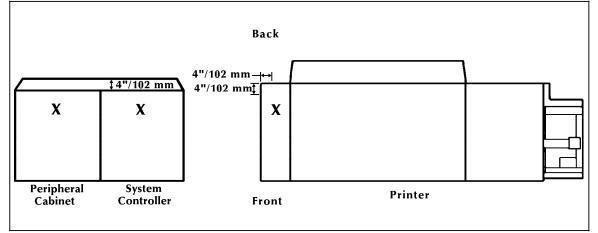
On the optional peripheral cabinet and the controller, the power cords enter from the bottom rear of the frames. The opening is in the middle.
