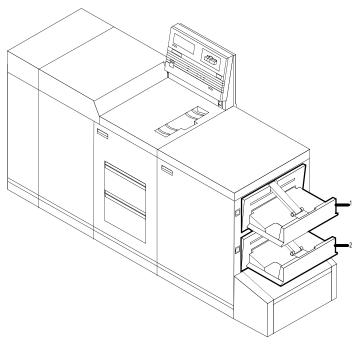
Figure 3-3. DocuPrint 4050/4090 NPS dual stacker configuration
