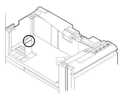
8. Pull the length guide forward to touch the back of the paper stack.
