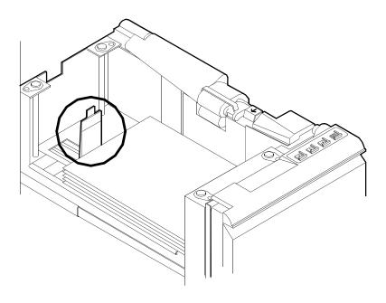
Latch the paper feeder assembly by pressing the green dot next to the green release lever until the assembly clicks into position.
