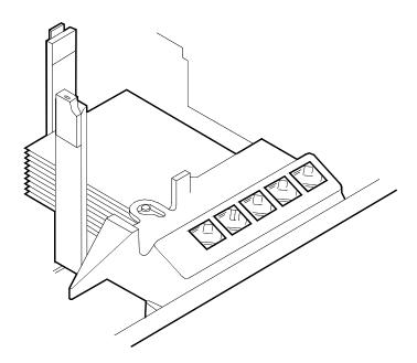
NOTE: The way you load the paper depends on the paper size required by the job. For paper longer than 14 inches, load the long edge against the back guide.
