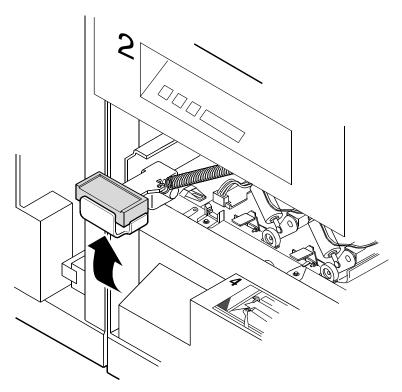
3. Locate the Q850 sensor and gently wipe the sensor with a dry cleaning pad.
