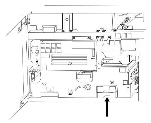
2. Place a dropcloth on the floor under the dry ink waste container area.
