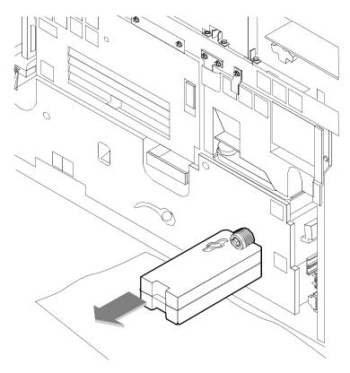
4. Remove the cap from the top of the full container and screw the cap onto the mouth of the container.
