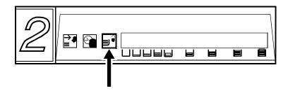
NOTE: If the printer has stopped due to a low paper condition, you do not need to press the Tray Unlock button.
