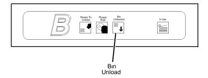
Once a bin is selected, the bin elevator lowers and the bin cannot be used until it is emptied completely. When the bin elevator stops in the down position, the Ready to Unload indicator lights.
