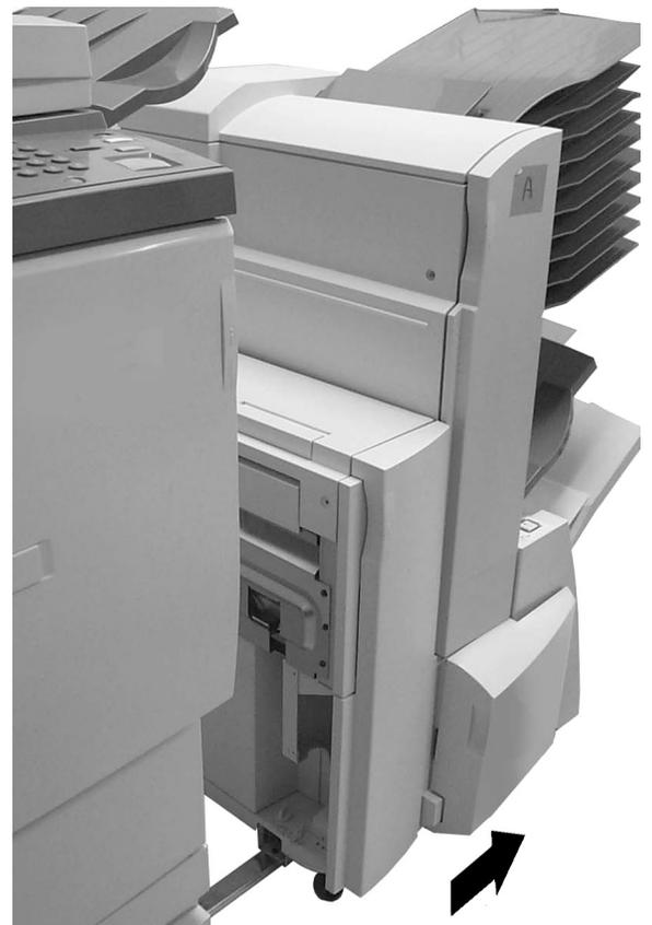
**Figure 9: Moving the Finisher away from the copier/printer**
