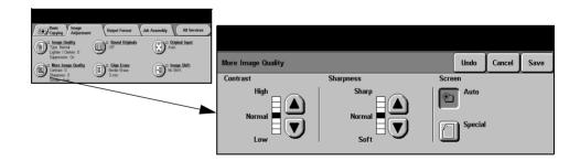
CONTRAST This option controls the differences between the image densities within the copy. Select a lower setting to improve the copy quality of pictures. Select a higher setting to produce more vivid blacks and whites for sharper text and lines.
