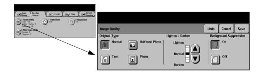
ORIGINAL TYPE Use this option to enhance the quality of the fax based on the type of original being scanned.
