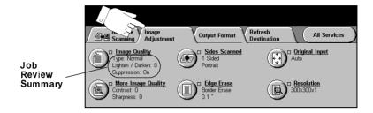
Touch any of the top level buttons to select a feature. To view all the options for a feature, select the feature required. Multiple options can be selected for each scan job if required.
