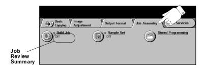
Touch any of the top level buttons to select a feature. To view all the options for a feature, select the feature required. Multiple options can be selected for each copy job if required.
