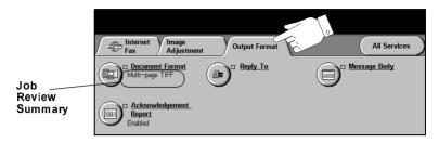
Touch any of the top level buttons to select a feature. To view all the options for a feature, select the feature required. Multiple options can be selected for each fax job if required.
