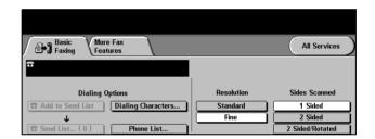
The *Basic Faxing* tab is the default screen for the Fax function. Use this tab to enter the recipient telephone number and to select the standard features for a fax job.
