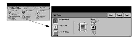
BORDER ERASE Erases equal amounts on all edges of the copies. Up to 2.0 inches in 0.05in. increments can be erased.
