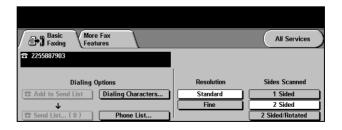
ADD TO SEND LIST Used when you want to send a fax to more than one destination. Enter the number using the keypad or select the *Phone List* button and select a stored number. Then select the Add to Send List button. Continue to add numbers until all the locations have been entered
