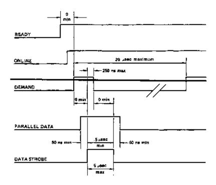
The data transfer rate is contingent upon the DATA STROBE being raised within 1 microsecond after DEMAND and dropped within 5 microsecond s. DEMAND may stay low longer than 20 microsecond s if a fault occurs or the 4235 LPS buffer (512 bytes) is full.
