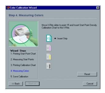
1. Insert the Image Density calibration chart into the X-Rite autoscan densitometer as shown in the illustration below. Begin with the cyan column.
