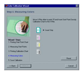
**1.** Position the X-Rite DTP34 over the Image Density calibration chart and follow the scan sequence as prompted.
