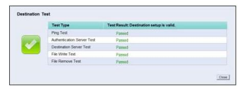
**Caveat:** If using IPV6 addresses, the Scan Destination Test available on the Embedded Web Server will incorrectly fail its Ping test even though the IPv6 address works in an actual scan if all other settings are correct. For Scan Destination Test purposes please use either the hostname or an IPV4 address.
