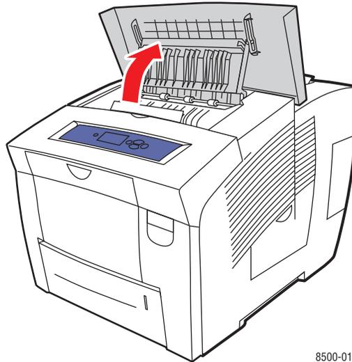
2. Pull the jammed paper slowly out of the printer. Confirm that any torn pieces of paper are removed.
