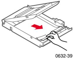
4. Close the Duplex Unit; press down to make sure that it snaps shut on both sides.
