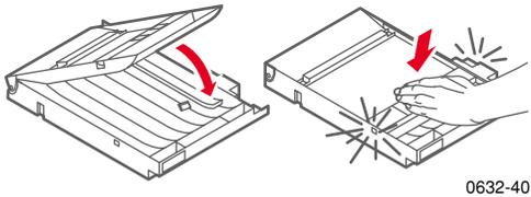
5. Re-insert the Duplex Unit into the printer's *upper* slot.
