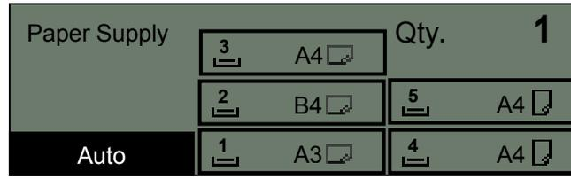
**Step 4** – Once you have selected a feature, the **Arrow** buttons are not usable. Use **Select** buttons again to choose your option. To move up and down a column of options press the **Select** button directly beneath the option you want (e.g. press third **Select** button twice to choose Tray 5). Press the **Enter** button to complete selection.
