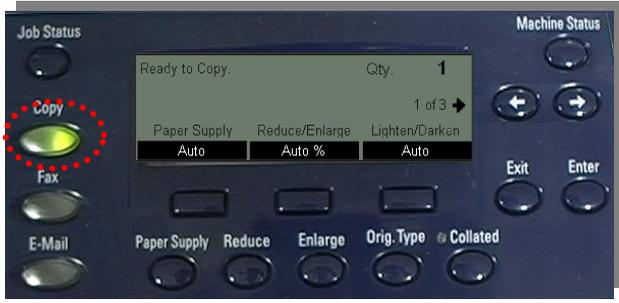
**Step 1** – Press the **Copy Mode** button on the control panel to access the Copy screens.
