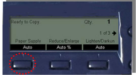
**Step 3** – Press the **Select** button directly beneath the feature you want (e.g. Paper Supply).
