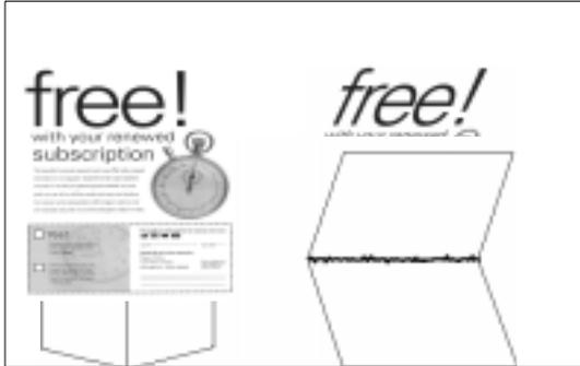
One method used to determine the grain is to fold a sheet of paper lengthwise, then make a crosswise fold. Compare the two folds. Paper folds smoothly with the grain. Cross-grain folds tend to be rough and cracked.
