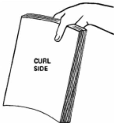
If the wrapper on a ream of paper is not marked with an arrow showing the wire side of the paper, the side of the paper facing the seam of the package is the wire side. Or, you can determine the curl side by holding a one-half inch stack of paper by one of the short edges.
