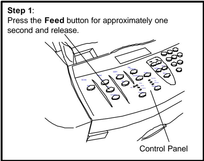
Figure 2. Pressing the Feed Button
