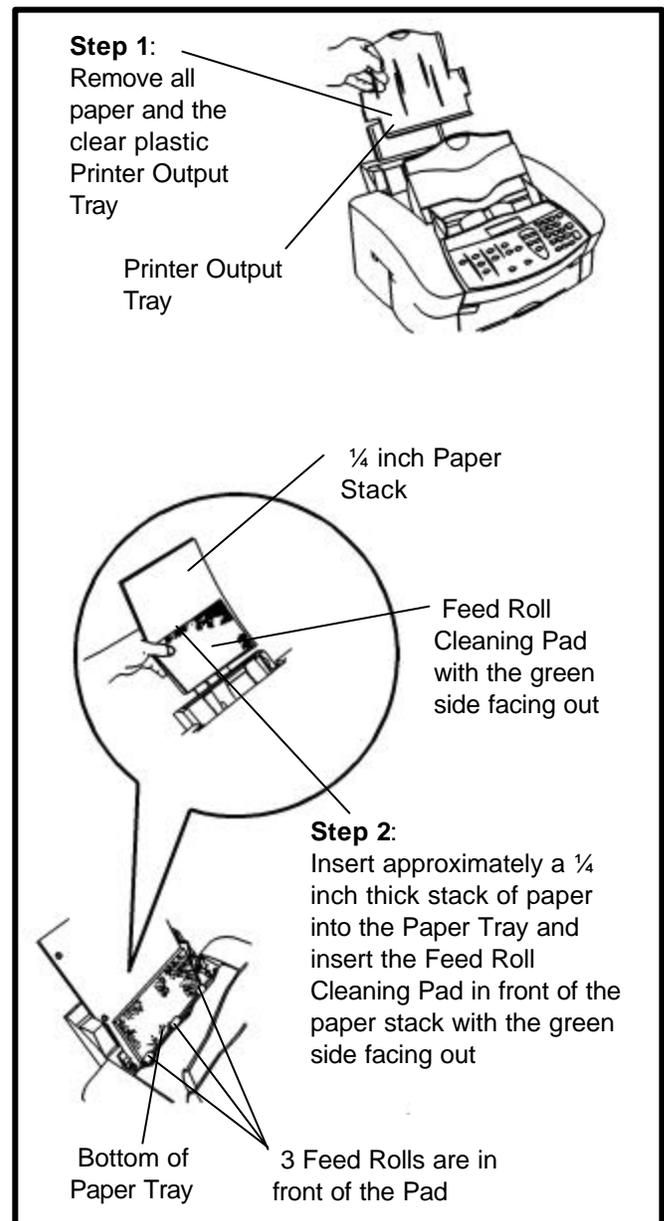
Figure 1. Inserting the Feed Roll Cleaning Pad into the Paper Tray
