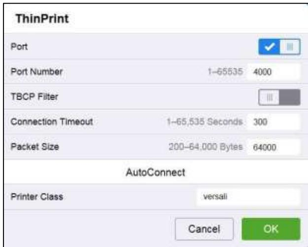
ThinPrint requires a certificate to be loaded on the device when running with TLS encryption. This is located in System Security SSL/TLS Settings
