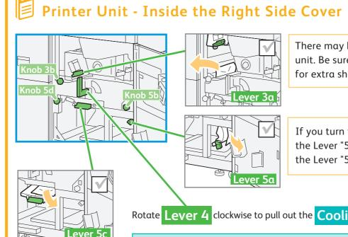
There may be extra sheets remaining in the printer unit. Be sure to turn the knob at least 3 times to check for extra sheets.
