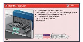
Attention is required to remove jammed papers in the part where 1 is displayed. Please read the instructions well and remove the paper.
