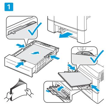
For best results, fan the edges of the paper. Adjust guides to fit the paper size. Do not load paper above the maximum fill line.
