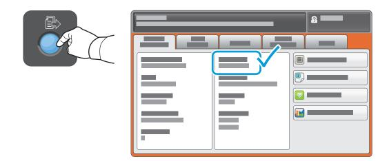
If the IP Address does not show in the upper left corner of the touch screen, press **Machine Status** and check the information field.
