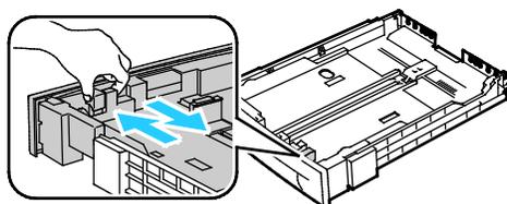
4. To compress the tray for shorter paper, with one hand, hold the back of the tray. With the other hand, at the front of the tray, press the release latch, then push the ends inward until they latch.
