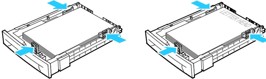
**Note:** Do not load paper above the maximum fill line. Overfilling the tray can cause the printer to jam.
