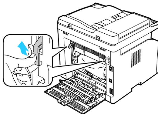
3. To remove any jammed paper from the back of the printer, carefully pull it in the direction shown.
