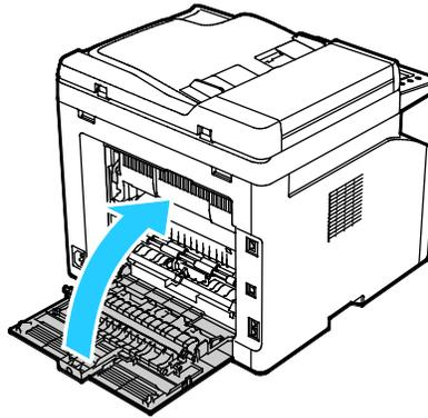
7. To resolve the error displayed on the control panel you must clear all paper from the paper path.
