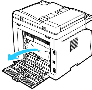
4. If you cannot find the jammed paper in the paper path, remove any jammed paper from the output tray.
