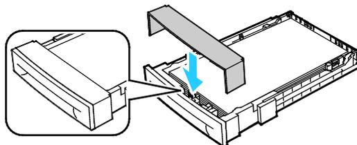
6. Load paper into the tray, then insert it back into the printer.
