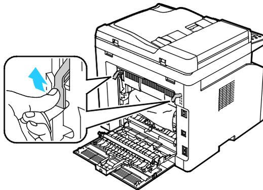
3. Remove any jammed paper from the back of the printer.
