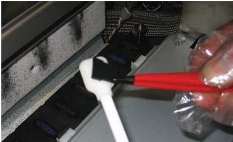
6. Standing in front of the printer, hold the wiper as shown on the image below.
