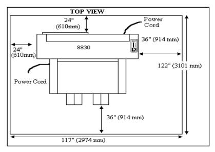
**Floor space requirements:** With printer: 122 inches x 117 inches (3101 mm x 2974 mm)
