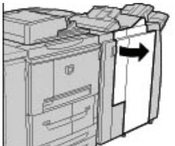
2. Pull out the tri-fold output tray 2d, swing lever 2g to the right, and remove the jammed paper.
