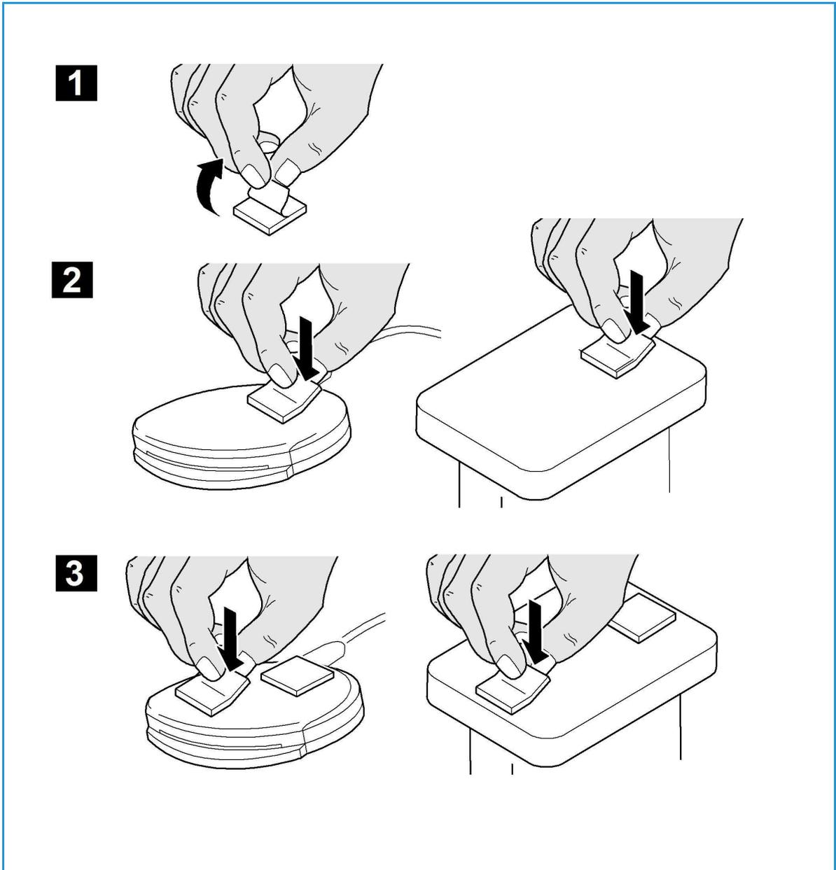
5. Remove the fastener backing strips
