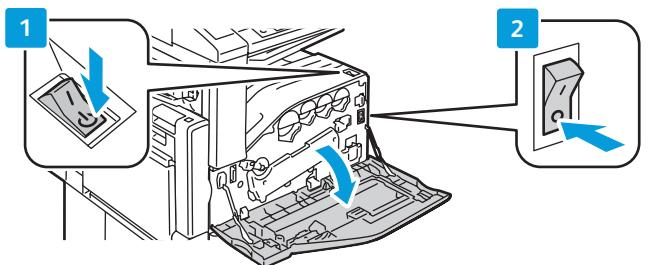
**EN** To restart printer, use **power switch** on top of printer. For full shut down turn off **power switch**, then turn off **main power switch** behind front cover.
