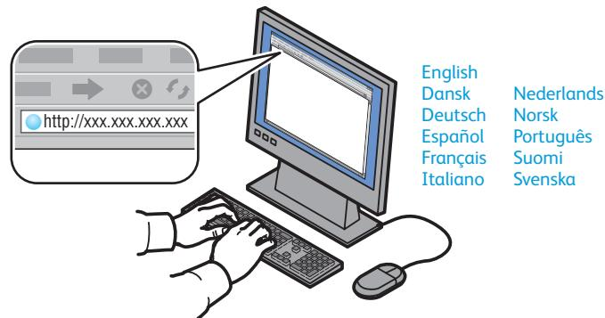
**EN** CentreWare Internet Services enables you to access printer configuration, security settings and diagnostic functions, and to manage address books and scanning over a TCP/IP network. To connect, type the printer's IP address in your computer's Web browser. The IP address is available on the Configuration Report information page.
