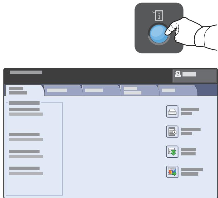
**EN** The Machine Status menu provides access to supplies status, printer information, and settings. To access all menus and settings, log in using the administrator name and password.
