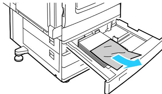
6. Verify that the paper is loaded correctly in the tray and that the guides are pressed firmly against the paper.
