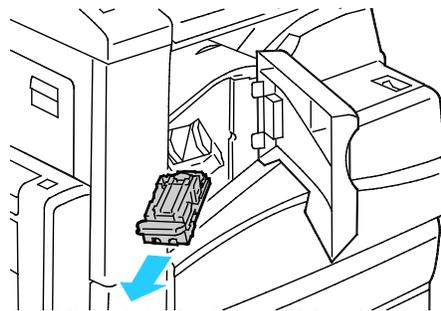
3. Remove any loose staples or other debris from inside the finisher.
