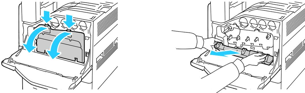
5. Remove the laser window cleaning wand from inside the front door.
