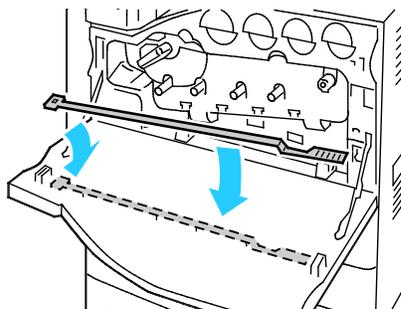
8. Align the bottom of the waste container with the tabs.
