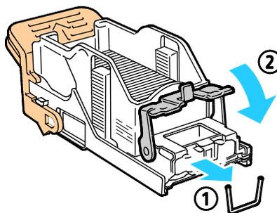
5. Grip the staple cartridge by the orange handle and insert the cartridge into the stapler until it clicks.
