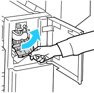
4. Grip the staple cartridge by the orange handle and pull it firmly toward you to remove it. Check inside the finisher for any loose staples and remove them.
