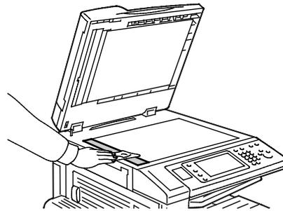
2. Use a lint-free cloth and Xerox® Cleaning Fluid to clean the underside of the document cover and the document feeder.
