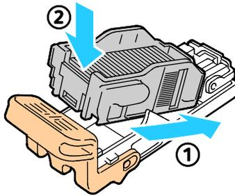
6. Grip the staple cartridge by the orange handle and insert the cartridge into the stapler until it clicks.
