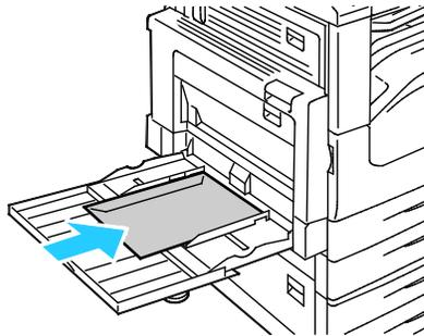
4. Adjust the width guides to fit the envelopes.
