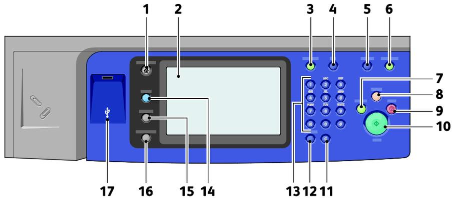
1. **Services Home** provides access to printer features, such as copy, scan, and fax, on the touch screen.
