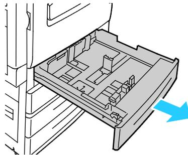
2. Ensure that the guide locks are set in the correct position for the size labels you are loading. For details, see [Setting the Guide Locks in the 500-Sheet Adjustable Trays](#) on page 59.
