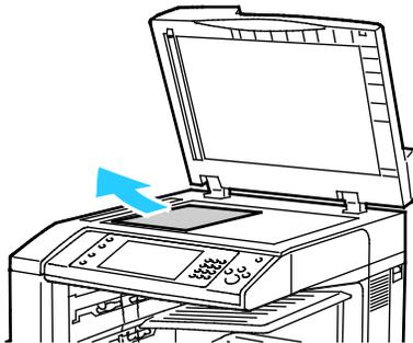
8. If the original is not visible when the document cover is opened, lift the document feeder tray, then remove the paper.
