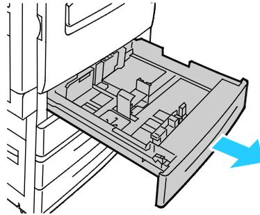
2. Load the envelopes in the envelope tray with the flaps closed, flaps down, and on the leading edge, toward the left.
