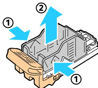
5. Insert the front side of the new staple case into the staple cartridge (1), then push the rear side into the cartridge (2).
