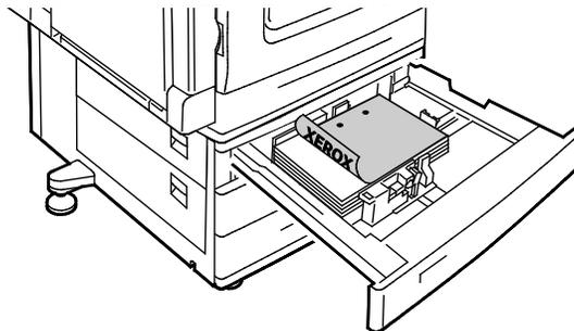
**Note:** Do not load paper above the maximum fill line. Overfilling the tray can cause the printer to jam.
