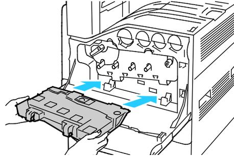
9. Rotate the waste container up, toward the printer until it clicks into place.
