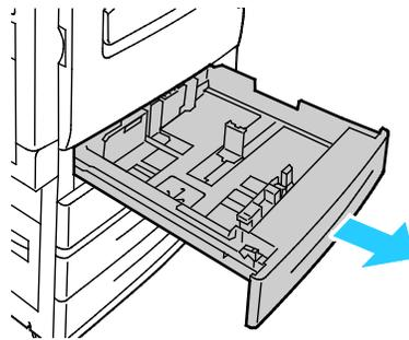
2. Ensure that the guide locks are set in the correct position for the standard or custom size paper you are loading. For details, see [Setting the Guide Locks in the 500-Sheet Adjustable Trays](#) on page 59.
