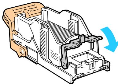
9. Grip the staple cartridge by the orange handle and insert it into the stapler assembly. Push it in until it clicks.
