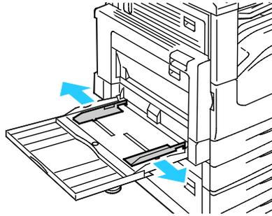
3. Load the envelopes face down with the flaps closed:
