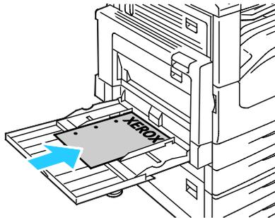
**Note:** Do not load paper above the maximum fill line. Overfilling the tray can cause the printer to jam.
