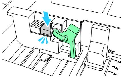
5. Load the custom-size paper in the tray. The tray guides move in 1 mm increments.
