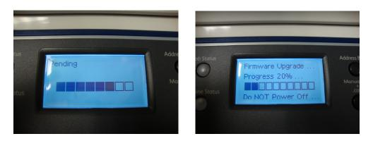
5. Once the upgrade is complete, you can remove the USB flashdrive. The machine will return to ready mode briefly, then reboot once, and return again to ready mode.
