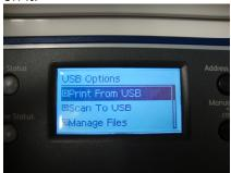
3. Press the **Up/Down** arrow buttons until the Upgrade **[.hd]** file you want is highlighted (see example below) and press **<OK**>.
