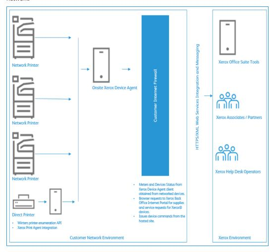
Figure 1: Typical Xerox Device Agent Deployment
