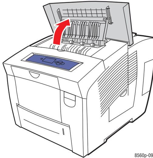
2. Lift the lower paper guide toward the front of the printer.
