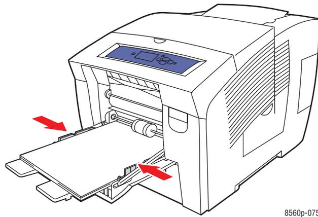
5. On the control panel, press the **OK** button if the correct paper size and **Labels** are displayed as the current setup, or select the label size and type:
