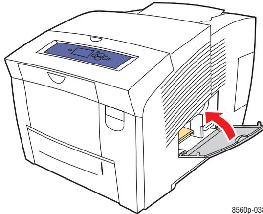
**Caution:** Do not attempt to reuse the waste ink in the printer; it can damage the printer. This damage is not covered under the printer warranty.
