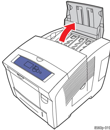
3. Locate the ink-loading bin that is low. A label above each bin indicates the ink stick color and shape for that bin.
