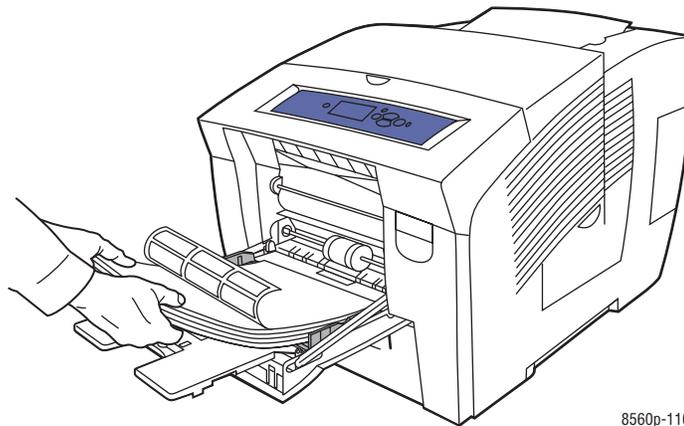
4. Adjust the paper guides to fit the labels loaded in the tray.
