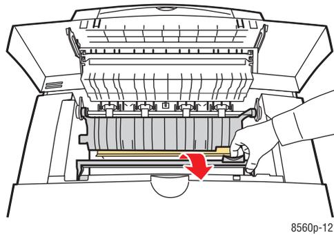
3. Wipe the plastic paper release blade on the lower paper guide with a pre-soaked alcohol cloth (using 90 percent isopropyl alcohol).
