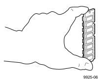
7. Insert the card into the slot, aligning the notches with the ridges in the slot. Press firmly. The white tabs will snap into place, locking the card in the slot.
