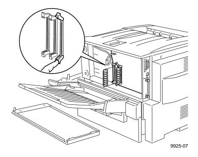
**6**. Hold the memory card by the edges with the **notched** long edge toward the printer.
