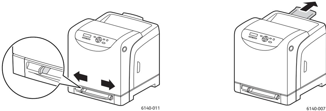
2. Open the output tray to hold the printed sheets.
