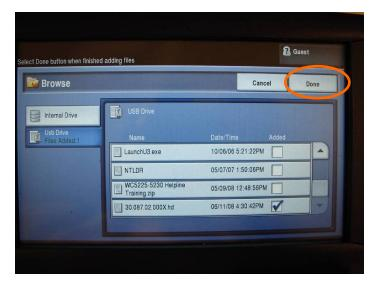
6. Select the Upgrade File [.hd] by touching it. Press the green **<Start>** button on the front panel to send the file to the machine and start the upgrade process.
