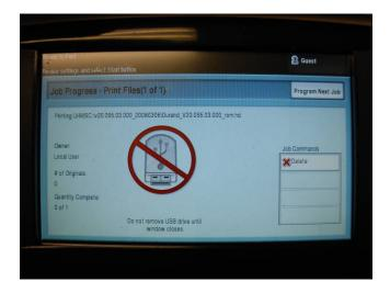
8. The User Interface will then go blank for a minute then indicate the status of the upgrade. It is now safe to remove the USB thumb drive. It will take approx. 25 minutes to finish the upgrade. The machine will reboot once the upgrade is complete.
